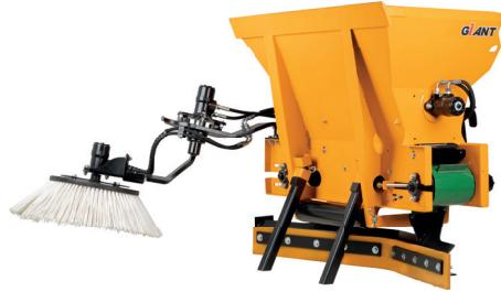
These divide buckets ZV come standard with stirring auger at the top, left and right discharging and dosing plates above conveyor belt. The necessary connection for this attachment demands 1x double-acting hydraulic function.
