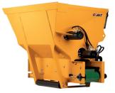
These dividing buckets MVB are equipped as standard with stirring auger at the top, an auger at the bottom, left and right discharging and dosing plates above conveyor belt. The necessary connection for this attachment demands 1x double-acting hydraulic function.
