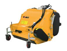
These flail mowers with collector come standard with paddle flails pressed steel of 3 mm thickness. The required connections for this attachment demands 2x double-acting hydraulic function, 1x single-side hydraulic hold, 1x free hydraulic return and 1x leak oil connection.
