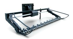
These cutter bar mowers are standard equipped with a rotating hitch and ground following by using slotted holes,. The necessary connection for this attachment demands 1x double-acting hydraulic function + single side hydraulic hold, pro inching and on recommendation a tandem pump + free hydraulic return.
