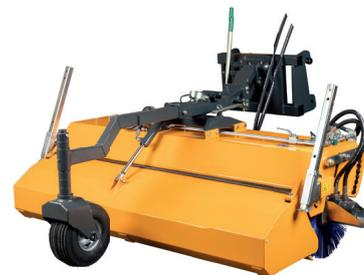
These sweepers plus come standard with level compensation system, 20° mechanical angle adjustment and a height-adjustable sweeping brush with premium brush quality. Also, this attachment has an XL running wheel with pneumatic tire height adjustment, hydraulic emptying and 3D levelling.
